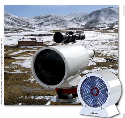
The Scintec BLS450 Large Aperture Scintillometer measures atmospheric turbulence and heat flux over path lengths between 250 m and 6000 m. As part of a meteorological station it can also be used to determine the evapotranspiration over extended areas.
